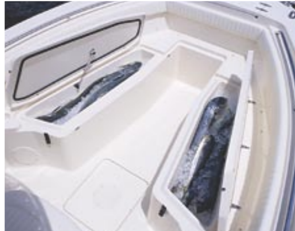
Bow fish boxes convert to bow seats (optional casting platform insert available)
