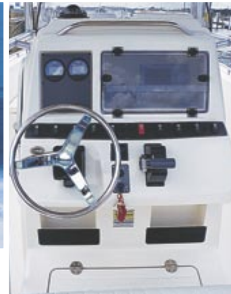
Helm station with lockable electronics box
