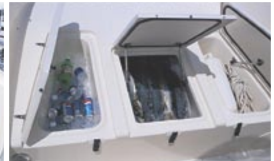
Insulated bow fish boxes with overboard drains
