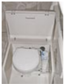
Head area in lockable cabin, with fold down cover; optional electric marine head shown
