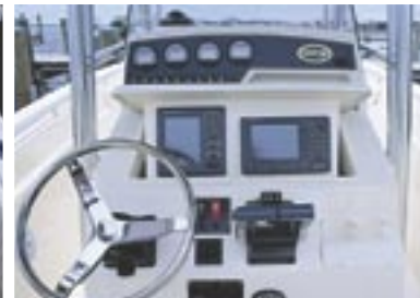
Helm console with electromechanically operated lockable electronics enclosure
