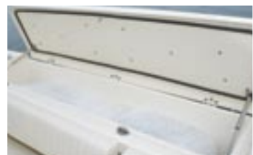
254-qt. aft deck insulated fish box
