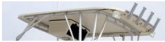
▲ Hardtop with lockable radio box, spreader lights and rod holders (208)
