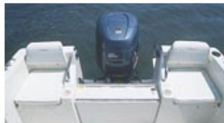
Aft cockpit with fold down motorwell bulkhead
