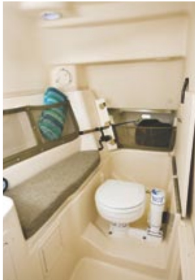
Stand up head area with bulk storage; fold down head cover creates 5' berth.
