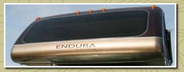
**Automotive Style Window** and mounting system creates a low maintenance aerodynamic, sleek modern appearance on the exterior. (Not Available with cabover entertainment center.)
