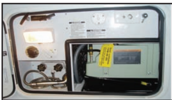
Centralized utility center includes drain valves, city water hook-up, outside shower, black tank flush, 12 volt master disconnect and Cable TV and satellite TV hook-ups
