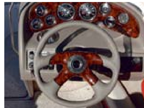
Helm with S/Steel bezels and digital depth sounder w/outside air and water temperature.
