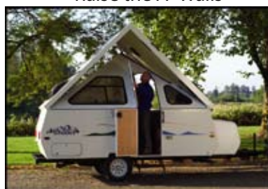
Raise the A- Walls
