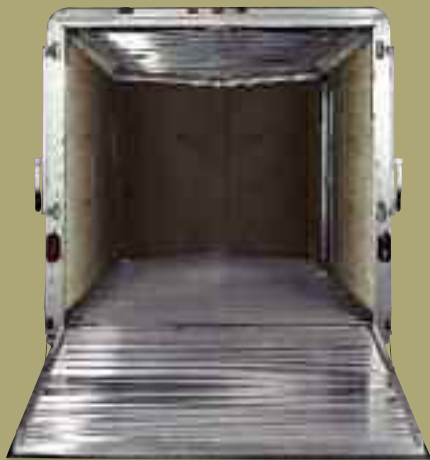
Precision crafted all aluminum welded roof truss construction • Crossmembers 16" on center
