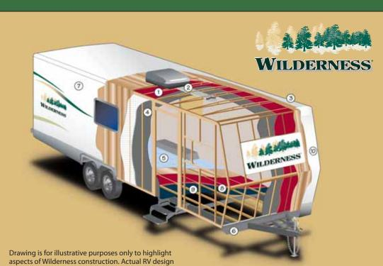
1. ENGINEERED RADIUSED CEILING TRUSS - Helps to ensure strength, water runoff and reduced
