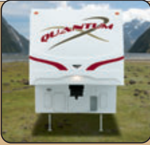
THE FRONT CAP gives the Quantum a smart profile, made from molded fiberglass.
