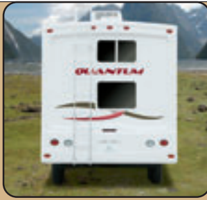
THE REAR CAP is made of molded fiberglass for an attractive rear view.
