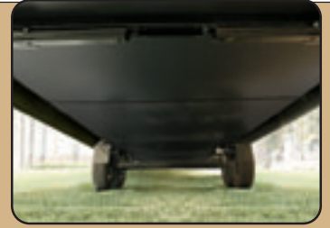
A FULLY ENCLOSED CHASSIS is available. No need to migrate to warmer climates. The enclosed chassis allows heating the holding tanks to help prevent freezing in colder weather.
