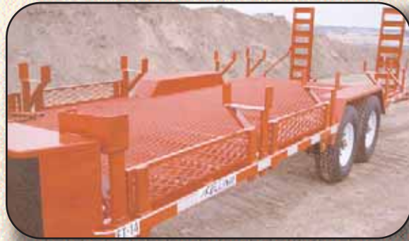
RACKS FOR PIPING
