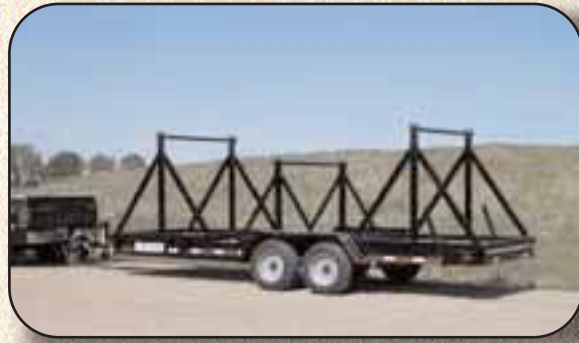
FT-16DE WITH REEL RACKS
