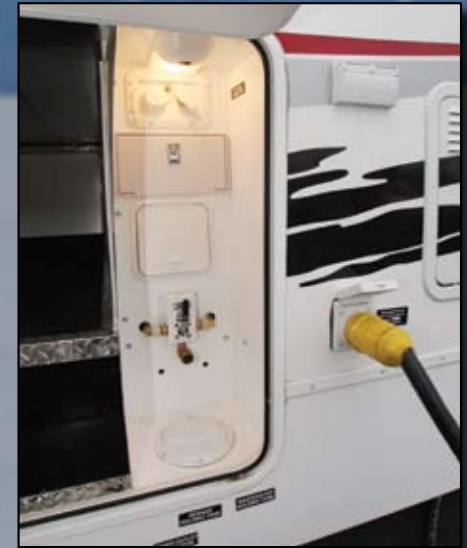
Centralized shore hookups with exterior shower
