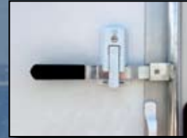
Anti-theft bar with lock on rear ramp door
