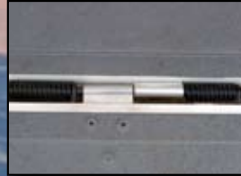
Hinge integrated springs on ramp door
