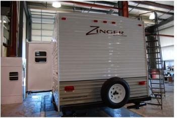
Now the graphics & awning are installed, cabinet doors are installed and the entire interior is trimmed and cleaned. Each unit is weighed and a label is placed on the interior side of the passage door.
