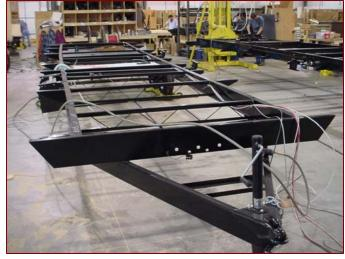
The Zinger's powder coated frames are built by Lippert™ Components. 6" I-Beam is used on non slide units, 8" is used on super slide units, and 10" is used on double slide units. The axles, jacks wiring & slide systems are installed in this station prior to floor installation.
