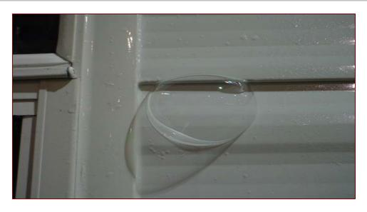
After the unit is pressurized and sprayed down with soapy water, bubbles will appear at any area that is not well sealed. These areas are then re-caulked and tested again before the unit is approved for shipment to the final owner.
