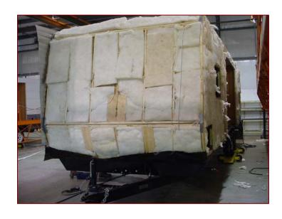
R-7 insulation battens are attached to the walls using a tacky wall glue to keep them from sliding in transit. The same system is used to insulate the roof prior to installing the roof.
