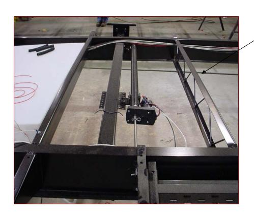
Note: The webbed I-Beam helps to reduce the overall weight of the unit.
