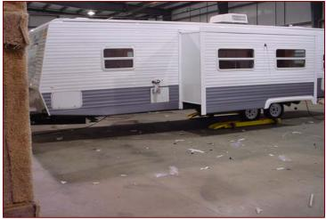
The siding, roof and slides are now installed. All metal is screwed, then caulked to protect the unit from leakage. Windows and door openings are cut out and these components are installed. Then the unit is ready for trim & graphics.
