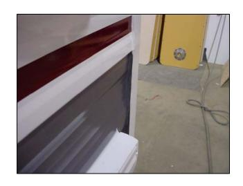
The entire unit is now sealed with polyurethane caulk to prevent leakage. Caulk is applied at every mating line & at every area where the skin of the unit has been cut, & at every corner.
