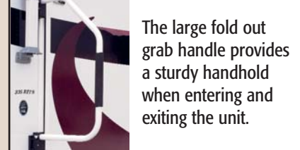
The large fold out grab handle provides a sturdy handhold when entering and exiting the unit.
