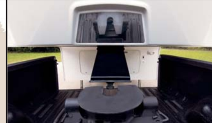
A cap mounted mirror gives you a solid view of the hitch from inside your truck for a confident hookup.
