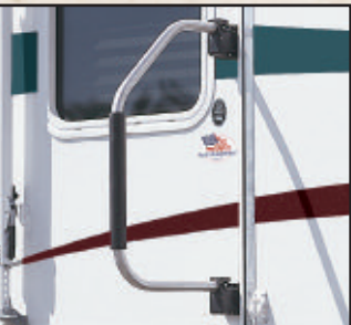
The large fold out grab handle provides a sturdy handhold when entering and exiting the unit.
