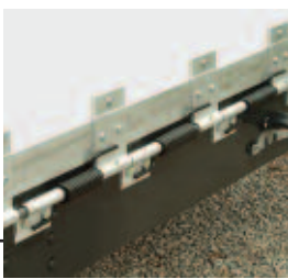
The cargo door features heavy duty, steel coil hinges designed to support the ramp when opened or closed, while eliminating the need for exposed cables and springs. Radius corners on the ramp door improve strength and a Grip Star™ ramp surface provides sure footing rain or shine. When its time to head out, the posi-lock latches provide a tight door seal. Integrated locks keep your toys secure and eliminate the need for padlocks.
