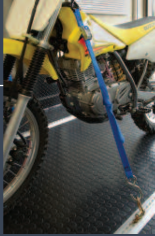
Adjustable track style tie downs line the cargo floor area allowing you to decide where to secure your toys.
