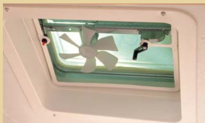
A 14" x 14" skylight roof vent with 12V fan is standard in all Dutchmen bathrooms.
