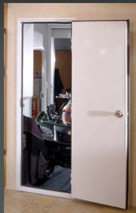
Sealed Cargo: Many models feature a sealed rear cargo area. The security door and wall are insulated to protect the living area of your SRV.
