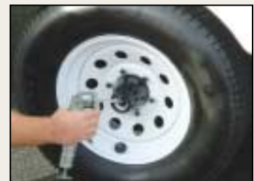
Ultra-lube hubs are standard on Denali. This feature allows for easy wheel bearing lubrication.
