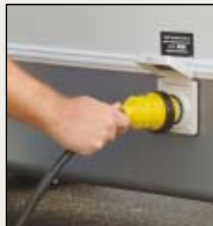
A 30 Amp marine grade detachable power cord stores in an outside compartment when not in use, saving valuable interior storage space.
