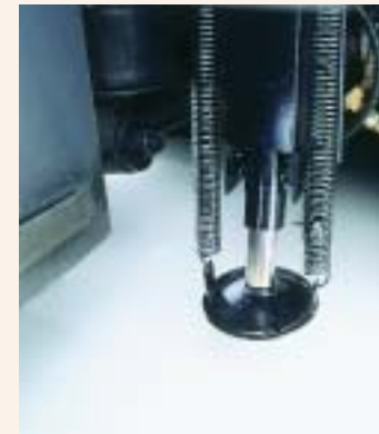
Four-point leveling jacks
