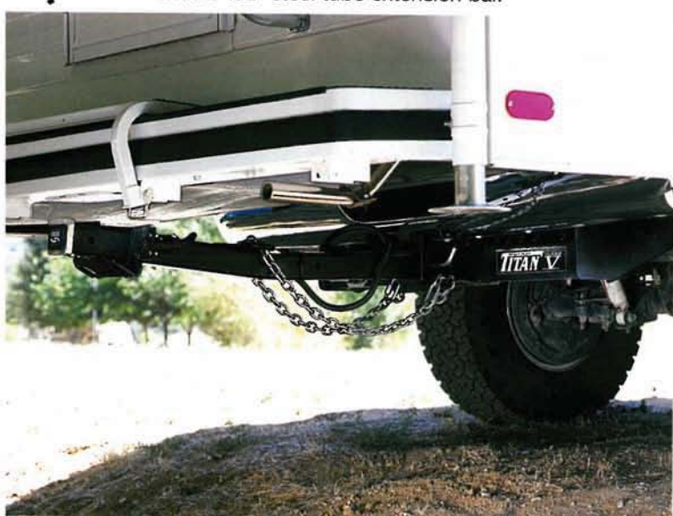
Reese TITAN Class V Receiver with 2-1/2" steel tube extension bar.
