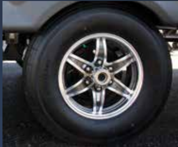
16" custom aluminum wheels with nitrogen-filled load range 'E' 10-Ply radial tires offer style and safety. Nitrogen reduces deterioration and helps maintain proper PSI over time.
