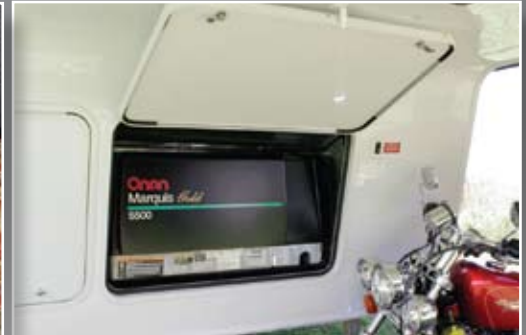
The Onan Marquis Gold Generator is noise rated for use after hours and comes with an automatic transfer switch!
