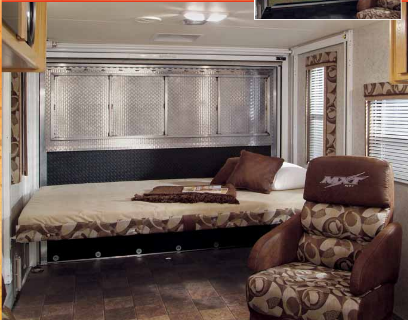
The optional rear door swings up and the loading ramp slides out from under the floor, providing a nice interior wall on the door as well as protection from the elements. Another thoughtful design from KZ Recreational Vehicles.
