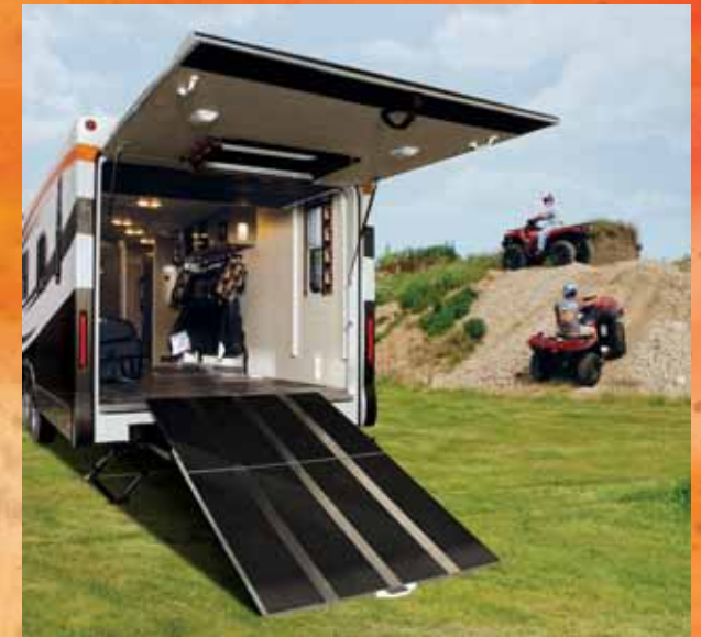
The optional rear door swings up and the loading ramp slides out from under the floor, providing a nice interior wall on the door as well as protection from the elements. Another thoughtful design from KZ Recreational Vehicles.
