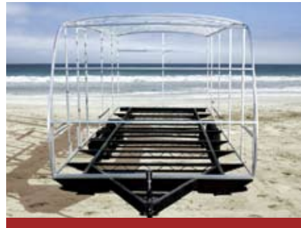
Coast features a crowned roof, aluminum structure and steel chassis for amazing stability
