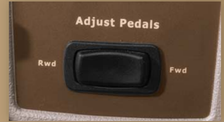
ADJUSTABLE PEDALS The automotive-style brake and accelerator pedals adjust at the push of a button.
