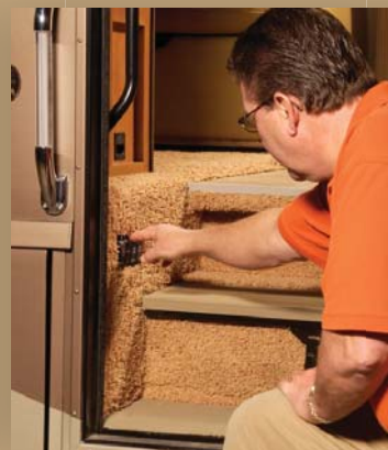
WEB POWERLINE ® Our energy management system monitors 110-volt electrical usage and automatically cycles postponable appliances on and off to prevent power overloads.
