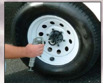
Ultra-lube hubs are standard on Denali. This feature allows for easy wheel bearing lubrication.
