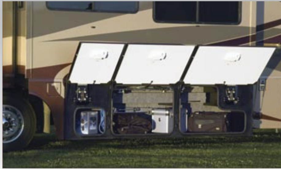
STOREMORE® The StoreMore slideout system allows exterior storage compartments to move in and out of the way when you need them.
